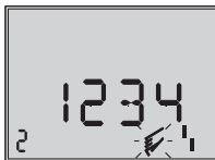
Reading direction for left attachment of pneumatic connections
