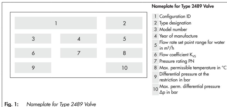
Fig. 1: Nameplate for Type 2489 Valve
