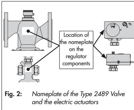
**Fig. 2:** *Nameplate of the Type 2489 Valve and the electric actuators*
